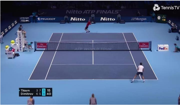
Figure 9: An HD (1920x1080 pixels) frame taken from a professional tennis match. The ball, positioned over the far tennis player, is nearly impossible to see from this resolution, making it difficult for a computer to perform essential training from this data.
